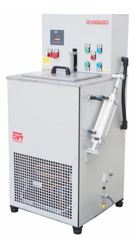
USED TO DETERMINE FLEXIBILITY OF BITUMEN SHEETS AT LOW TEMPERATURES
